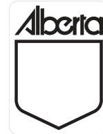
IB-2: Alberta route marker for highway numbers 1-216, NOT STOCK 45cm x 60cm, 60x75
